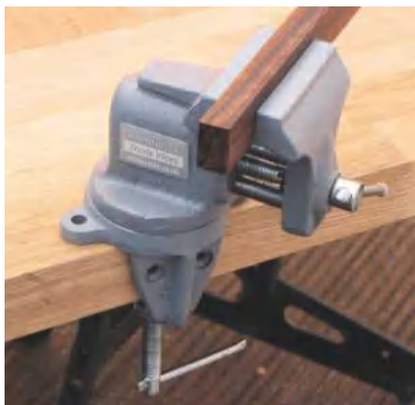
▲ A lower tommy bar enables you to attach the vice temporarily to a worktop up to 47mm-thick
